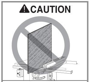
DO NOT place a tall board on edge to perform a rabbet cut with a standard blade. Workpieces that are too tall to be properly supported with the fence can easily shift during operation and cause kickback. Instead, place the stock flat on the saw and perform the rabbet cut with a dado blade.
